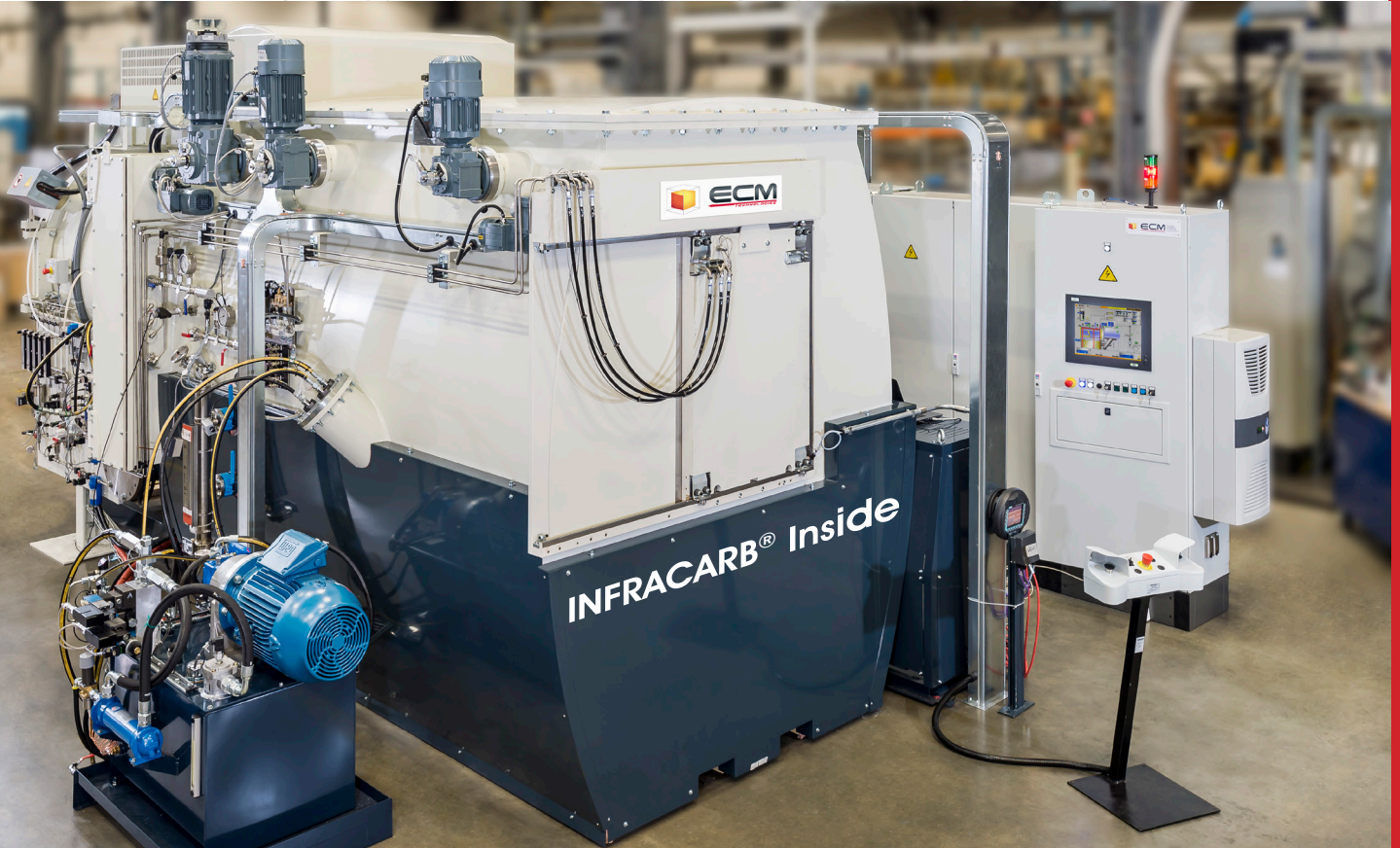
ICBP Duo® TH Oil Quenching pitless installation
